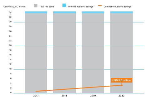
SFOC reduction 4g/kWh resulting fuel consumption savings of 1863.2 t/year
