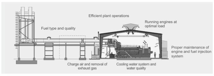
A site audit by energy efficiency experts helps identify equipment and processes with improvement potential. The power plant's technical schematics, designed operating parameters and available operational data are examined as basis for selecting the best improvement solution.
